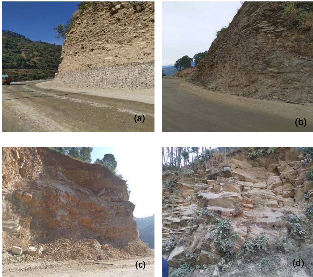
Fig. 9: Geological condition of the study area: (a)River Borne Material (RBM) unconsolidated form; (b) Phyllites, Metamorphic rock; (c) Hard and jointed rock is overlain by RBM; and (d) Slate/foliated metamorphic rock
