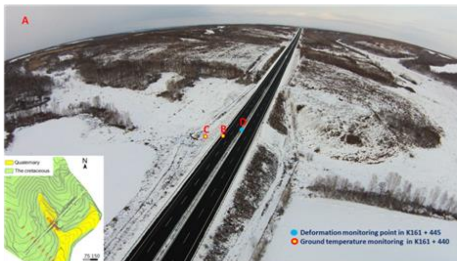
Figure 15.2. Measuring point position of Ground temperature and uneven settlement of the subgrade in K161+440 ~ K161+450 section during road operation
