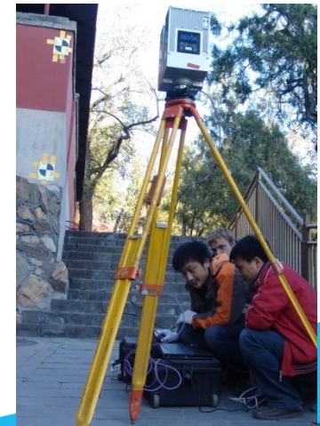
Researchers carrying out field work at the foot of Fo Xiang Ge using LIDAR technology
